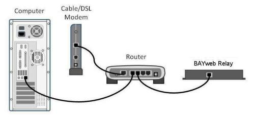
If direct wiring is not convenient, use Powerline Ethernet adapters. Plug one adapter into a power plug near the relay, and the other adapter near your router. Then just plug the Ethernet cables into the adapters and the ports as shown.
